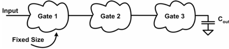
Figure 9-9. Chain of Gates with a Fixed Output Load and Fixed Input Size
