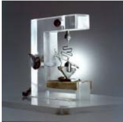
Fig. 1. The first contact transistor developed in Bell Laboratories by Bardeen and Brattain under the supervision of Shockley in 1948.
