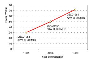
Fig. 1. Power increase for three generations of DEC "Alphd" processor
