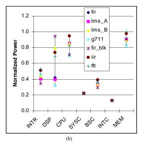
Fig. 2 Module-wise breakdown of the chip power consumption for the kernel benchmarks for the integrated RISC+DSP processor, (a) as a percentage of the total (b) normalized
