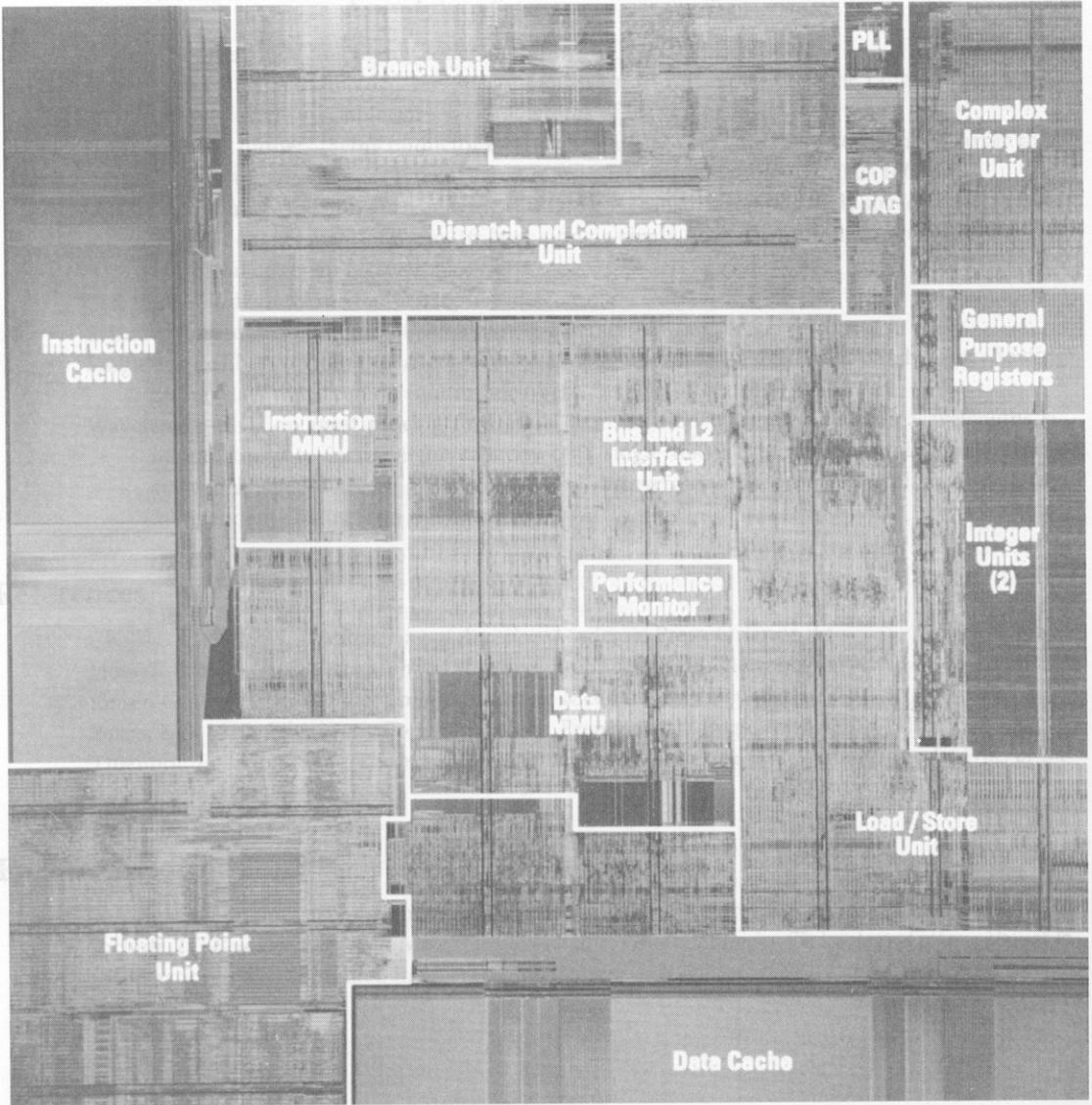
Microphotograph of IBM PowerPC 620™, a 64-bit super-scalar processor containing 7 million transistors and capable of issuing four instructions in a single cycle built in 0.5μ CMOS technology. The processor has 32 Kbytes of instruction and data cache memory, and employs register renaming and branch prediction mechanisms. It runs at 100 MHz and achieves 250 SPEC integer and 300 SPEC floating point operations. (Photo by Tom Way and courtesy of IBM.)
