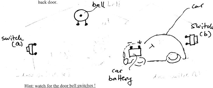
(b.) The door bell switch operates in the following way: when pressed the contact is ON. When released - there is no contact (it is OFF). What is the logical expression for the door bell as a function of the two door bell swithes a and b?
