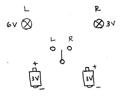
Problem 2: Complete the wiring diagram for the givven circuit. When the switch is in the L position the light L should be ON.
