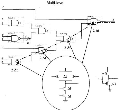
The path with the longest delay determines the speed of the network. In this case, the longest delay includes four 2 Input NAND gates, each with a maximum delay of 2  $\Delta t$  through the n-tree making the total delay through the network a maximum of 4 X (2  $\Delta t$ ) =  $8 \Delta t$  +  $1 \Delta t$  =  $9 \Delta t$
