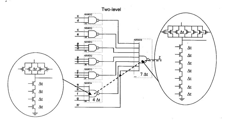
Again, the speed of the network depends on the slowest path. In this case, the gates with the highest fan-in are the slowest because adding more transistors to the gate adds more delay as shown above. The slowest path includes the 4 Input NAND gate which contributes a 4  $\Delta t$  delay and the 7 Input NAND gate which contributes a 7  $\Delta t$  delay making the total maximum delay through this network equal to 11  $\Delta t$ .
