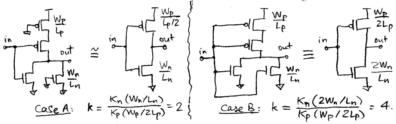
Assume PMOS and NMOS are identically sized such that  $\beta_p = \beta_n$ . That is,  $K_p (\frac{W_p}{L_p}) = K_n (\frac{W_n}{L_n})$ .
