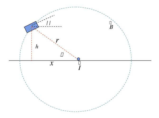
We would like to solve for S([], x, h, I), that is, our sensor output as a function of tilt angle, height, horizontal distance, and track current.
