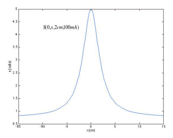
A tilt angle of 0 degrees shows a response that tails off as  $\sim 1/x^2$ .
