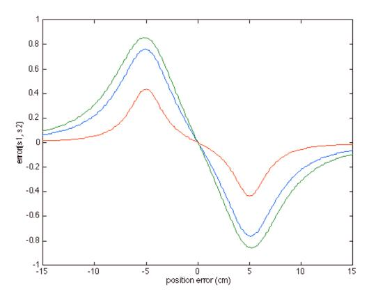
error<sub>green</sub> maintains its gain and maintains its linearity in the presence of half the track current.
