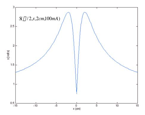
A tilt angle of 90 degrees has a null directly over the track, and tails off as  $\sim 1/x$ .
