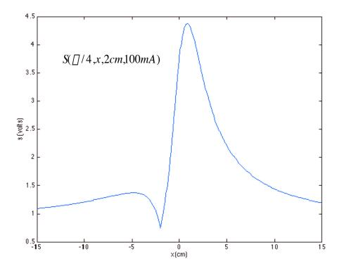
A tilt angle of 45 degrees allows differentiation between the two sides of the track.
