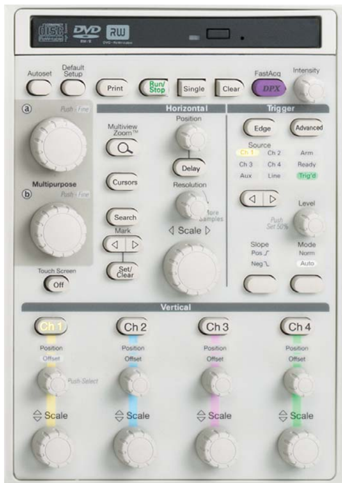
Figure 22. Front-panel control section of an oscilloscope.
