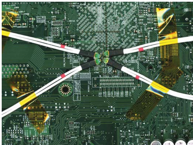
Figure 40. Dense devices and systems require small form factor probes.
