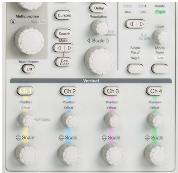
Figure 60. Traditional, analog-style knobs control position, scale, intensity, etc. — precisely as you would expect.
