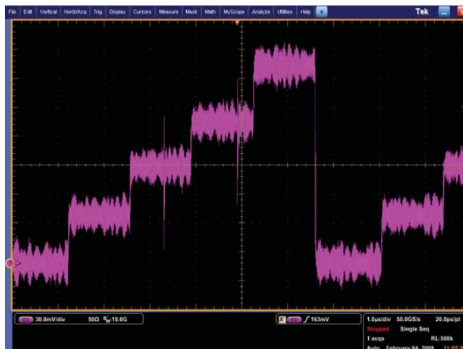
Figure 27. Peak detect mode enables the DPO70000B Series oscilloscope to capture transient anomalies as narrow as 20 ps.
