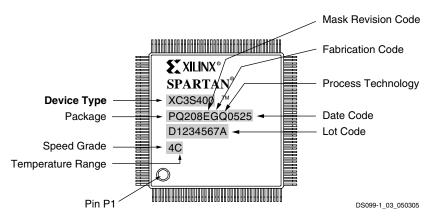
Figure 2: Spartan-3 QFP Package Marking Example for Part Number XC3S400-4PQ208C
