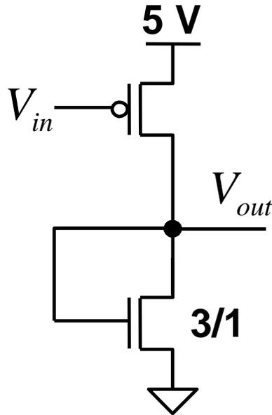
Figure 2: CMOS inverter.
