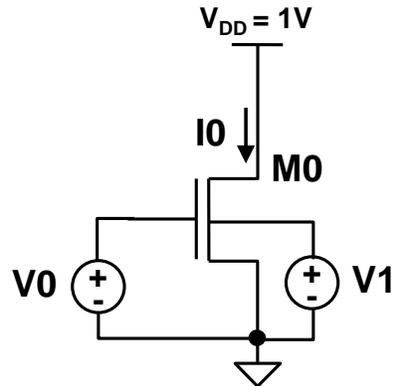
Figure 1: FET biasing circuit.
