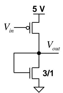
Figure 2: CMOS inverter.
