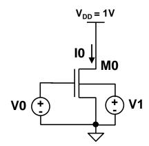
Figure 1: FET biasing circuit.
