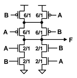
Figure 3: CMOS logic gate. All dimensions in microns.
