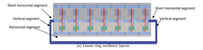
Method 1:  $T_{ring\ osc.} = 7 * \tau_{pd,inverter} + 7\ horizontal\ segments * \frac{2um}{segment} * \frac{14ps}{um} = 5376 + 196 = 5572ps;$
