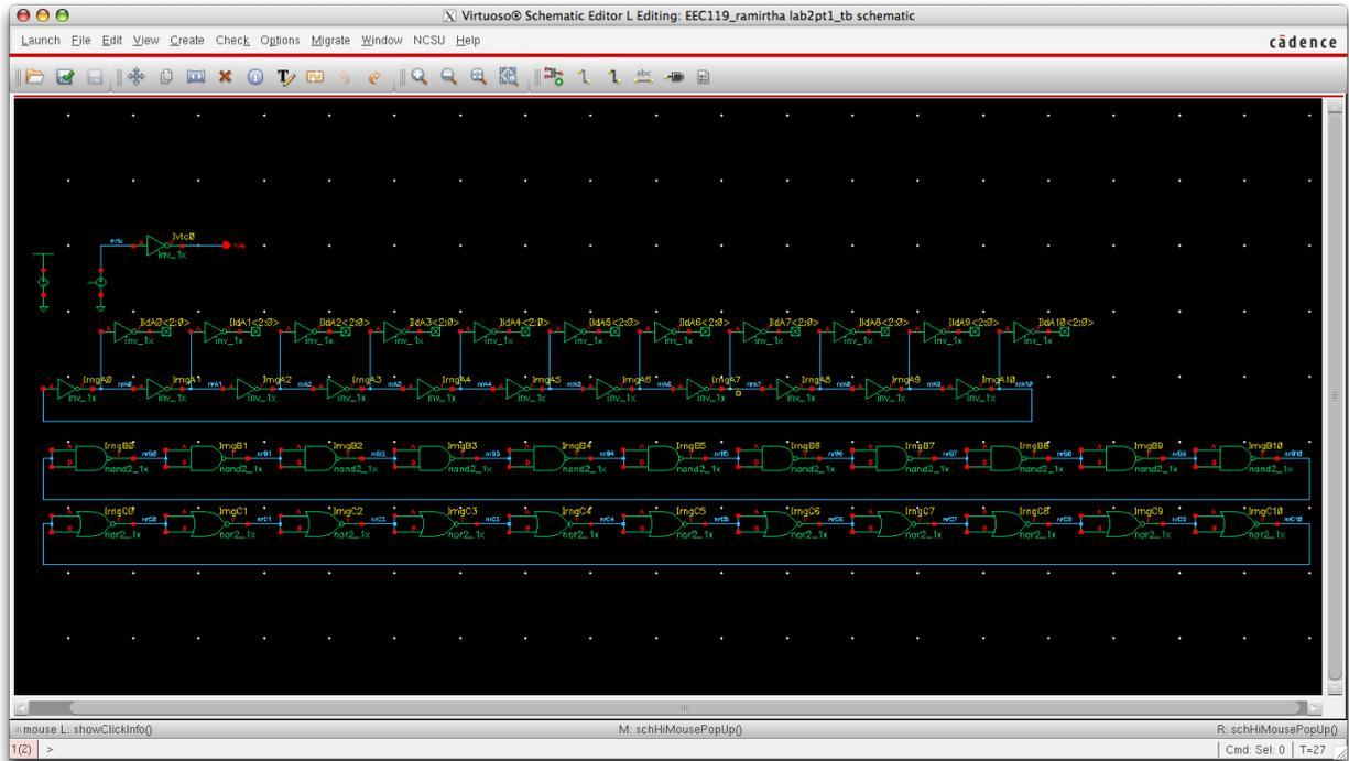
Figure 4: Three ring oscillator testbench schematic.
