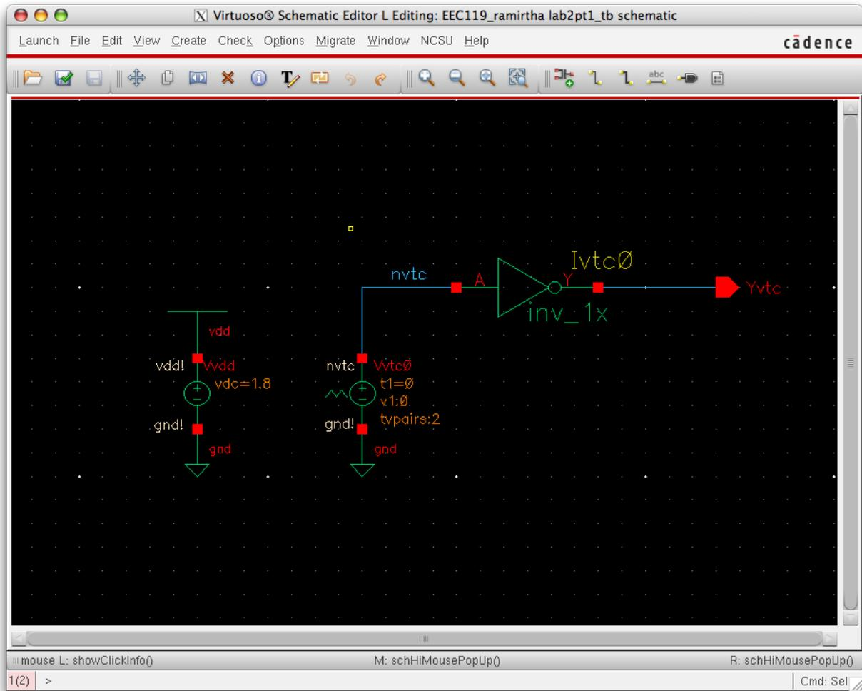
Figure 1: Inverter voltage transfer characteristic testbench schematic.
