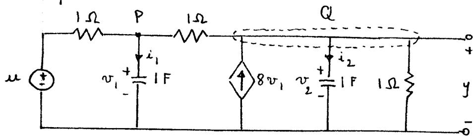
with initial conditions  $v_1(0) = 2 \text{ V}$ ,  $v_2(0) = 1 \text{ V}$ . Applying the KCL at points P and Q gives
