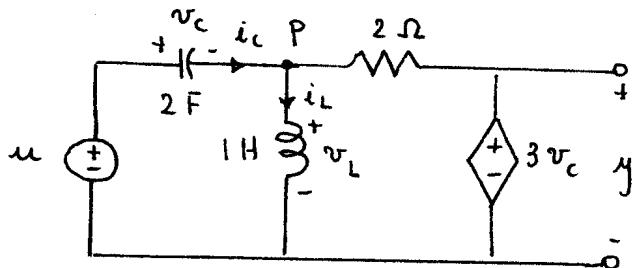
with initial conditions  $v_c(0) = 1V$ ,  $i_L(0) = 1A$ . The KVL along the left loop gives
