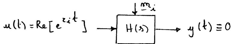
Thus, although we are exciting the system with the complex exponential input  $u(t) = \operatorname{Re}[e^{z_i t}]$ , nothing comes out! For this reason, the system zeros  $z_i$  are sometimes called transmission or blocking zeros.
