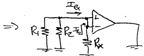
because of the high gain of the amplifier, we can assume a virtual short between input terminals:  $V_+ = V_-$
