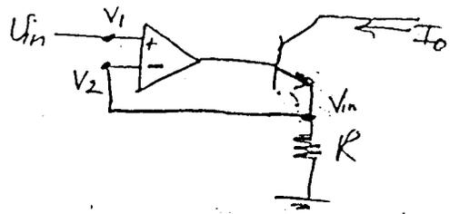
virtual short  $\Rightarrow V_1 = V_2 = V_{in}$
