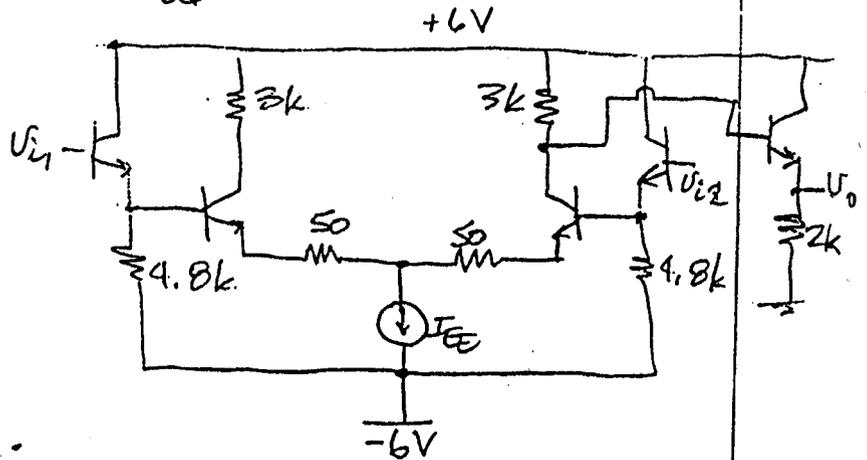
1st find gain of diff pair and then the gain of CE output stage and multiply together.
