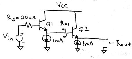
$$R_{\text{out}} = \frac{\Gamma_{\text{m2}} + R_{\text{ol}}}{B+1} = \frac{5.2k+124}{201} = 26 \Omega$$
