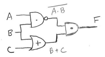
8. Draw a circuit consisting of AND, OR and INVERT logic gates that implements the function below. The inputs to the circuit are A, B and C.
