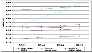
Figure 3. Break down of RF component delay with increasing RF size
