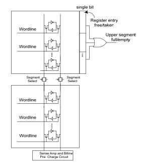
Figure 7. Proposed circuit modification for RF
