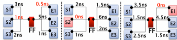
Figure 6. Timing slack transfer using CAT scheduling
