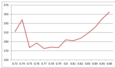
Fig. 10. Average latencies in clock cycles when the values of threshold 1 and 2 are adjusted (X-axis is threshold 1).
