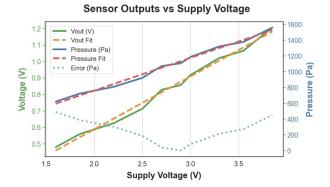
Fig. 7: Sensor output voltage, pressure reading, and pressure error relative to the original voltage of 2.9V (arbitrary), all as a function of the supply voltage. The slope of the dashed red fit regression line is 414.73 Pa/V and the slope of the dashed orange regression line is 0.321 V/V.
