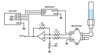
Fig. 5: Basic Hardware Schematic for Example Sensor Application. Only shows used pins on the nRF52 and MAX20303.
