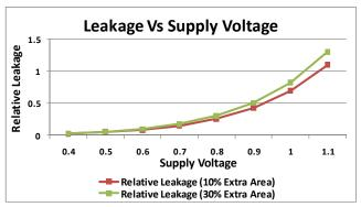
Figure 9: Relative Leakage for different supply voltages for SRAM
