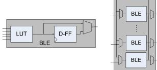
Figure 1: BLE (left) and CLB (right) structure in FPGA architecture
