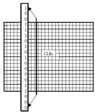
Figure 2: CLB Frame in Xilinx FPGA
