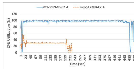
Figure 12(b): CPU utilization trace of Wordcount for number of mappers comparison
