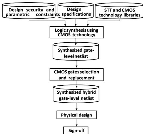
Figure 3. Our novel security-driven STT-CMOS hybrid design flow.
