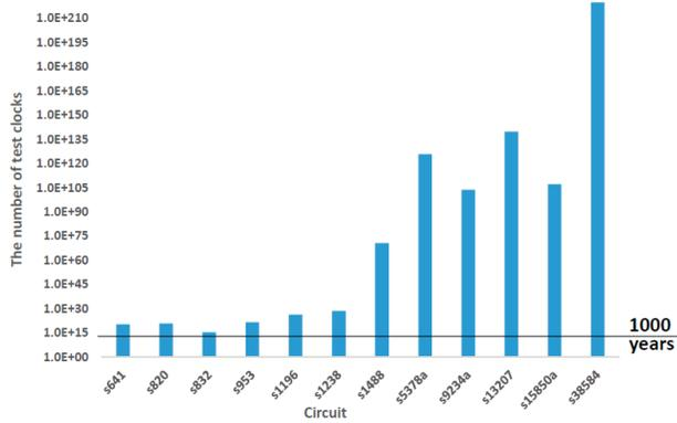
Figure 4. The number of possible required test clocks to determine the functionality of missing gates.
