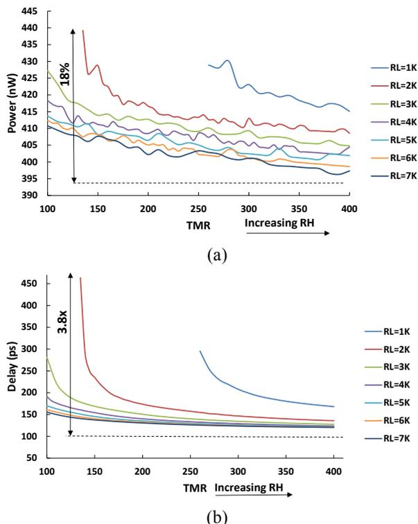
Figure 2. (a) Power and (b) Delay of STT-LUT vs TMR. RH and RL denote the high and low resistances (RAP and RP) of the MTJ.
