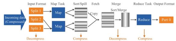
Fig. 1. Hadoop MapReduce: Computational Framework Phases [2].
