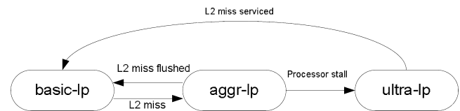
Fig. 18. State machine to control MZZ-HVS for DL1 (write port) and L2 cache.
