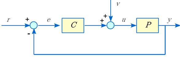
Fig. 1. Feedback Control System
