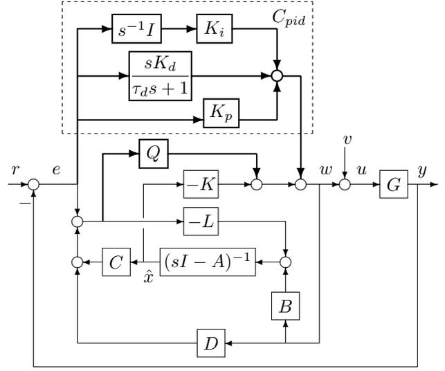
Fig. 3.  $Sys(G,\hat{C})$  using full-order observer-based controller  $C_g^o$
