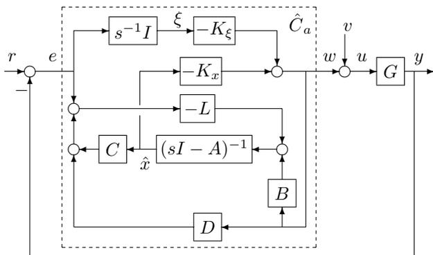
Fig. 4.  $Sys(G, \hat{C}_a)$  with augmented observer-based controller. 2594
