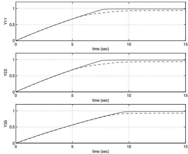
Fig. 6. Step responses of  $Sys(G, \hat{C}^o)$ ,  $Sys(G, \hat{C}_a)$  without integrators.
