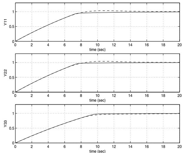
Fig. 7. Step responses of  $Sys(G, \hat{C}^o)$ ,  $Sys(G, \hat{C}_a)$  with limited integrators.
