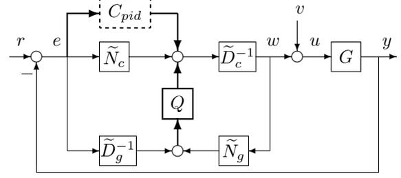
Fig. 2. The system  $Sys(G,\hat{C})$  with integral-action controller  $\hat{C}$ .
