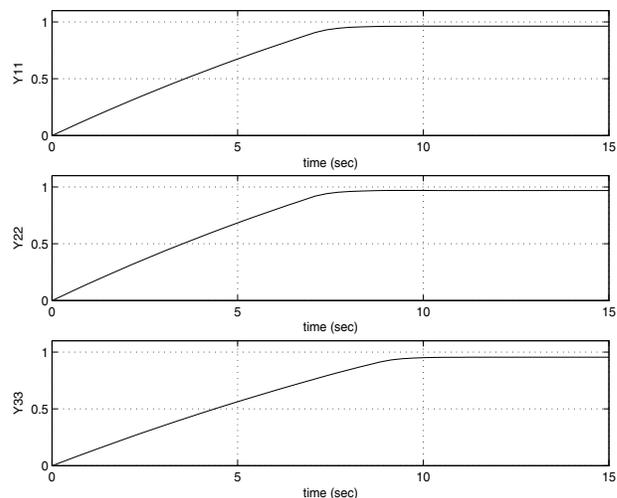
Fig. 8. Step response of  $Sys(G, C_g^o)$  with saturated input.
