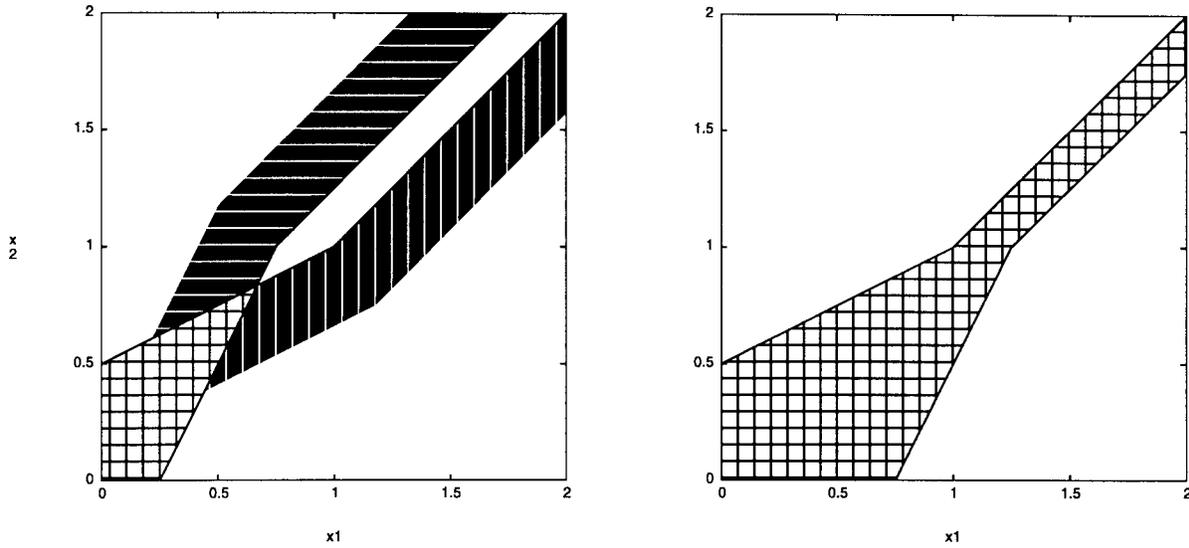
Fig. 2. Feasible regions for  $\alpha = [0.25 \ 0.5]^T$  and  $\alpha = [0.75 \ 0.5]^T$  for two identical piecewise-linear bounding functions: below  $(x_1, \alpha_2 + \varphi_1(x_1))$  and above  $(\alpha_1 + \varphi_2(x_2), x_2)$ . Changing  $\alpha_1$  corresponds to horizontal translation of  $(\varphi_2(x_2), x_2)$ .
