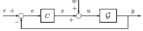
Fig. 1. The feedback system  $Sys(\mathcal{G}, C)$ .
