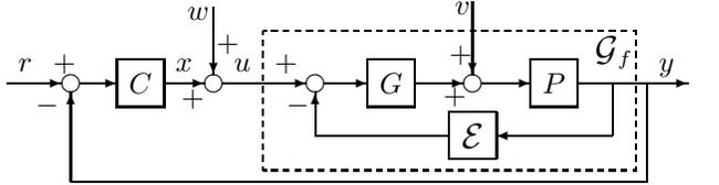
Fig. 4. The system  $Sys(\mathcal{G}_f, C)$  with interconnected feedback delay
