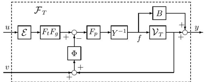
Fig. 6. Multi-area power system  $\mathcal{F}_T$  with a tie-line network  $\mathcal{V}_T$
