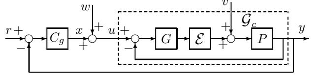
Fig. 3. The system  $Sys(\mathcal{G}_c, C_g)$  with interconnected cascade delay
