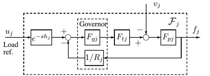
Fig. 5. Single-area power system with communication delay
