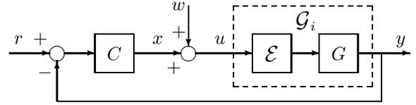
Fig. 2. The feedback system  $Sys(\mathcal{G}_i, C)$  with input delay in the plant
