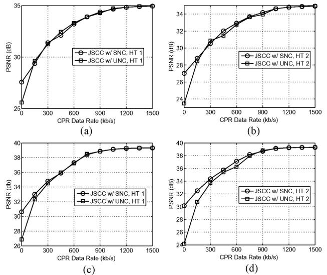
Fig. 6. Performance comparison between CPR-aware JSCC using UNC and SNC. (a) *Foreman* sequence, HT 1 loss. (b) *Foreman* sequence, HT 2 loss. (c) *News* sequence, HT 1 loss. (d) *News* sequence, HT 2 loss.
