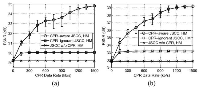
Fig. 4. CPR-aware rate-distortion optimized JSCC versus CPR-ignorant JSCC using UNC. WWAN loss rate 0.3. (a) *Foreman* sequence. (b) *News* sequence.
