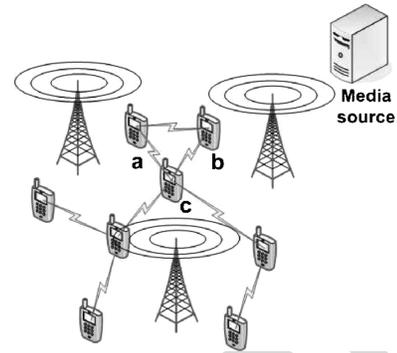
Fig. 1. Illustration of cooperative peer-to-peer repair network.
