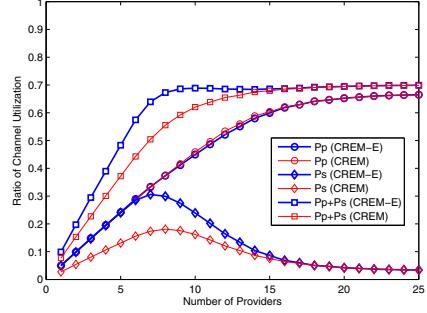
Fig. 3. Ratio of channel utilization vs. number of providers.
