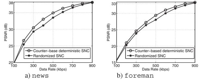
**Fig. 2.** Counter-based deterministic SNC selection with local optimization versus randomized approach.
