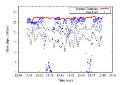
Fig. 3. The line plots show a snapshot of the normal performance template for network load along with the lower 3rd and 6th standard deviations. The scatter plot shows the raw data for the same time period for a different day.
