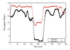
Fig. 1. Impact of two different scenarios on user throughput. Scenario 2 corresponds to an actual fault, while scenario 1 simply involves a new client being added into the network.
