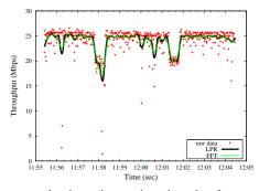
Fig. 2. The scatter plot shows the raw throughput data for a particular link in the wireless network. The line plots show the smoothed data that can serve as the template for normal network behavior.
