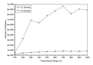
Fig. 3. Number of collisions observed for single source 10% and 30% scenario.
