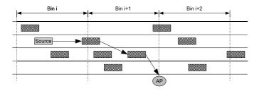
Fig. 1. A single source vehicle communicates with a fixed AP, using other vehicles as routers. The road is divided into bins consisting of 100 cells each.
