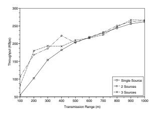
Fig. 8. System throughput of both single source multi-source with respect to transmission range in 10% traffic density scenario.
