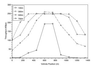
Fig. 5. Throughput for 30% density, correlated to vehicle position on the road. Position 0 in the plot corresponds to packets sent by the source when it is in cells 0-99(0-150 meters); position 100 corresponds to cells 100-199(150-300 meters).
