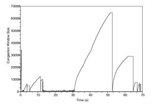
Fig. 9. Congestion window size as a function of time for a one of the 2 vehicle in the multi-source scenario. Vehicle density is 10% and transmission range is 100 meters.
