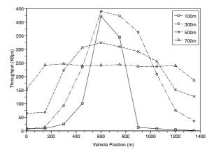
Fig. 11. Throughput of 3-source scenario at various transmission ranges. Vehicle density for this graph is 10%.
