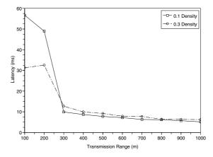
Fig. 4. Average latency from source to destination at 10% and 30% vehicle densities for single source.
