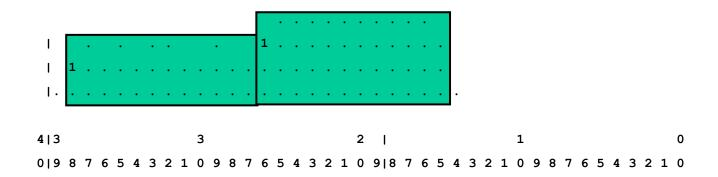
• After three levels of adders, it's ready for a carry-propagate adder!
