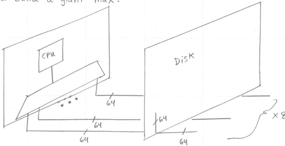
but the motherboard requires  $64 \times 8 = 512$  signal wires!
