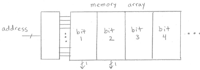
We can think of a ROM memory cell as a tri-state buffer: (enabled by decoder output)
