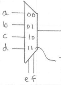
These values indicate which input is connected to the output when the control input(s) equal these values.
