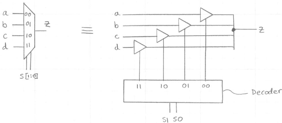
Ex: Suppose we need to communicate with one module at a time where there are from 1-8 modules. For example, on the PCI bus inside your computer:
