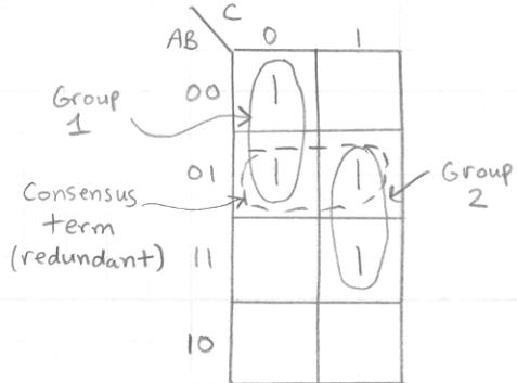
$$\begin{aligned} \text{Group 1: } A'B'C' + A'BC' &= A'C' \\ \text{Group 2: } A'BC + ABC &= BC \end{aligned} \quad \left. \right\} Z = A'C' + BC$$
