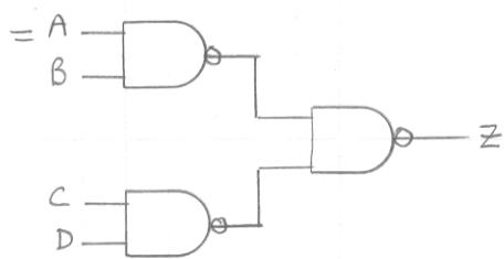
Ex: Write equation for the following circuit:
