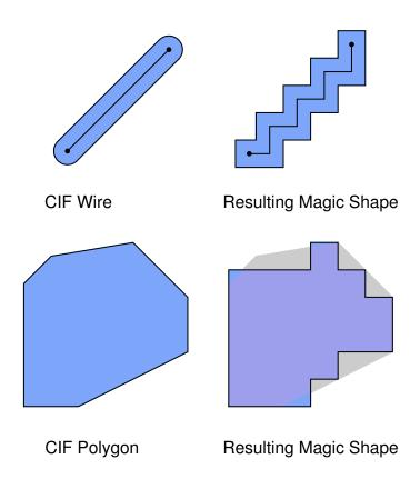
The shape of the Magic stairstep depends on the order in which vertices appear in the CIF or Calma file. The stairstep is made by first incrementing or decrementing the x-coordinate, then incrementing or decrementing the y-coordinate, then x, then y, and so on. For example, in the figure above, the polygon was specified in counter-clockwise order; if it had been specified in clockwise order the result would have been slightly different.
