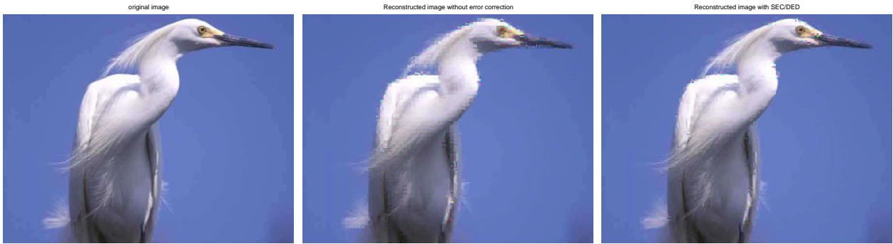
Figure 6: (left): original image;(middle): the reconstructed image without SEC for the code table; (right): reconstructed image with SEC/DED for the code table
