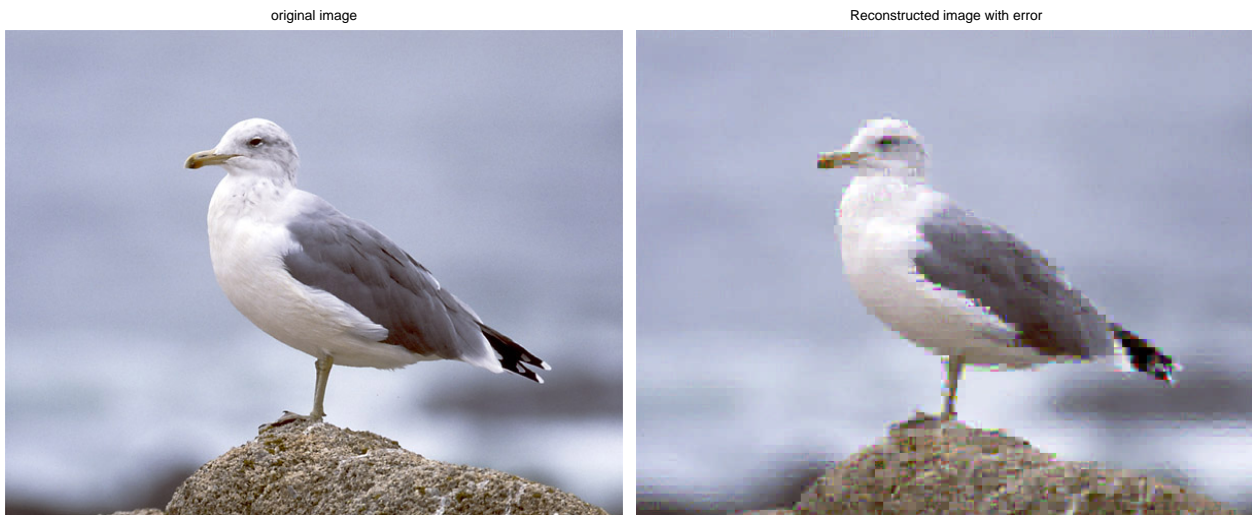
Figure 2: Original ( left ) and reconstructed ( right ) images under the memory fault effects. In this case, the error correction function was not activated. The coding for an 8 \times 8 DCT blocks is skipped when error is detected in the Huffman code table
