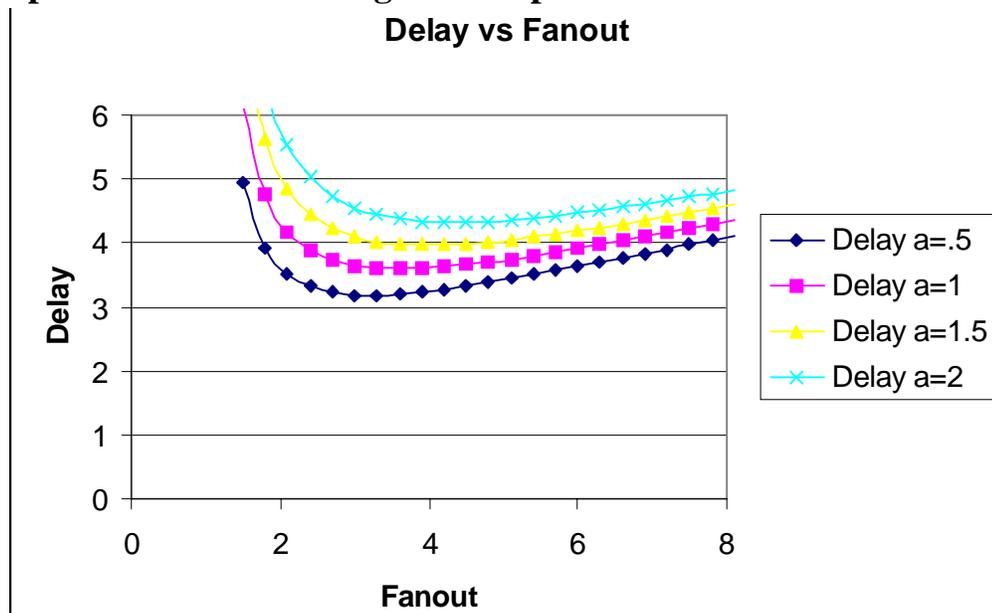
The question of the optimal fanout and number of stages in a chain, is both simple and a little tricky. This answer comes from solving the delay equation for a string of gates:
