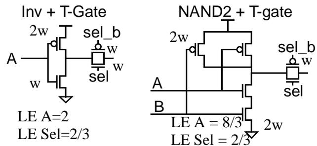
To get equal logical efforts, the resistance of the transmission gate must be made much smaller than the resistance of the inverter. Since the resistance of the supergate is the same for both inputs, to get equal logical efforts, we make the input capacitance the same. This makes the transistors in the TGate 3w for the inverter, and the LE of the both A and Sel 4/3. Obviously you can set the LE of the 'sel' input at any point in
