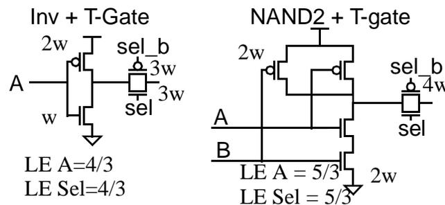
between these points. The ‘best’ LE depends on which of the inputs is critical. I don’t think it would make sense to go outside these two points, since both are getting a little inefficient in terms of making use of the transistor width consumed.
