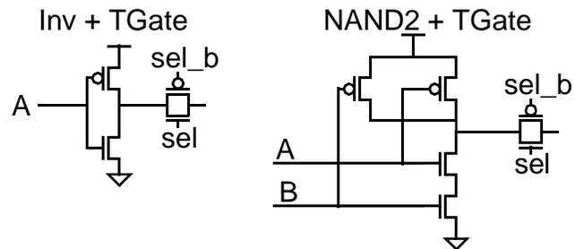
To start we need to know whether we should consider sel and sel\_b two different signals, or should we add the cap together. The answer is described in more detail in the next section, and turns out that the logical effort of a splitter (creates A and A\_b) is only slightly greater than one. So the logic effort should be considered by only looking at the 'sel' input.
