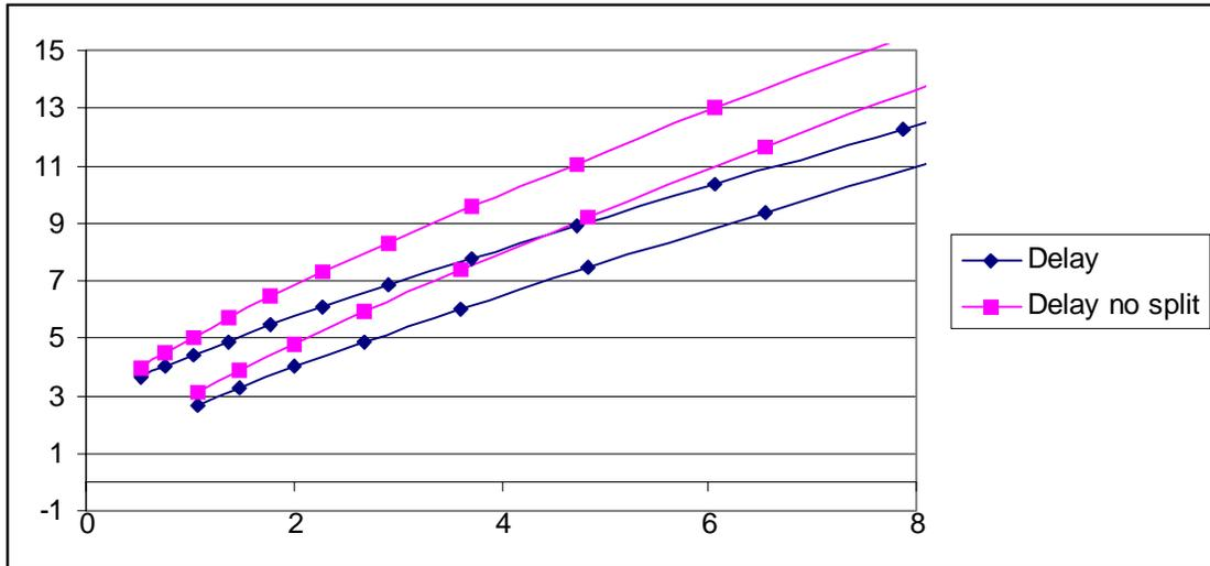
The blue curves (with diamonds) are the result of splitting the first inverter. If the inverter is not split (the first technique) you get the pink (squares) curves. The lower curves are the results you get if you ignore the parasitic delay, the upper curves are the results if the self loading is equal to its gate capacitance.
