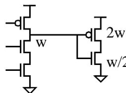
3). The LE for the two stages is .55, and the average LE per stage is 0.75. If we used a chain of these gates and tried to find the best fan out per stage, the answer would be that each stage should have an electrical fanout of about 4, (actually 4.4 for dynamic stage and 3.6 for the static gate). At this fanout, the effective fanout ( $LE * Fanout$ ) of the domino gate is 3, not 4.
