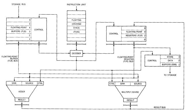
Figure 1 Data registers and transfer paths without CDB.
