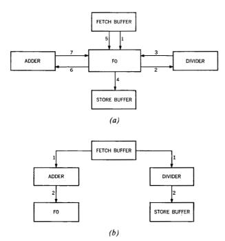
Figure 6 Functional sequence for Example 6 (a) with busy bit controls only, (b) with CDB.
