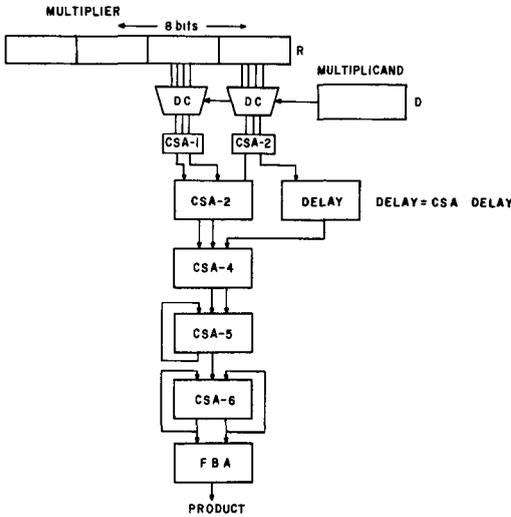
FIGURE 12f. Pipeline multiplication using 8-bit multiplier groups.
