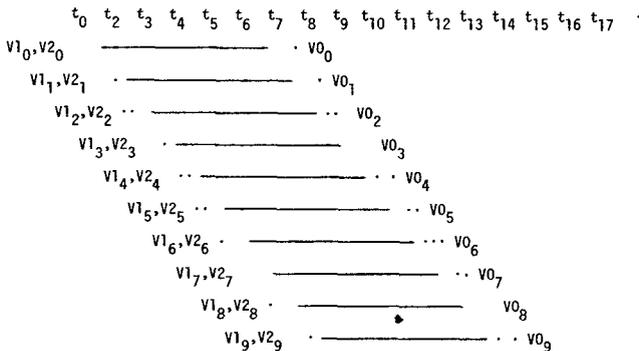
FIGURE 22. Vector instruction timing example ( $V_0$   $V_1$   $V_2$ ).
