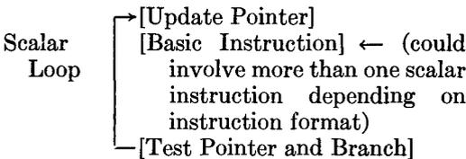
Execution of this loop  $L$  times requires considerable time. One significant factor is the operand fetch, which is not done (look-ahead) fast enough as in the vector counterpart. So, by the time the operand comes back from memory, several precious processing cycles have been lost (Figure 19).
