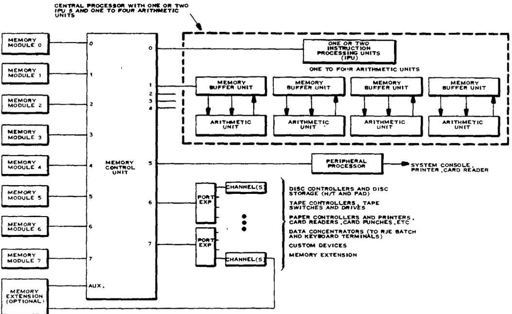
FIGURE 9. ASC system configuration.
