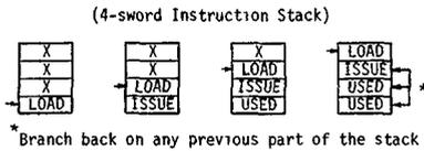
FIGURE 12a. STAR-100 instruction stack loading and issuing with branch tolerance.
