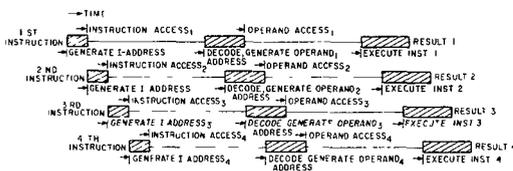
FIGURE 2. IBM 360 Model 91 instruction sequencing illustration.
