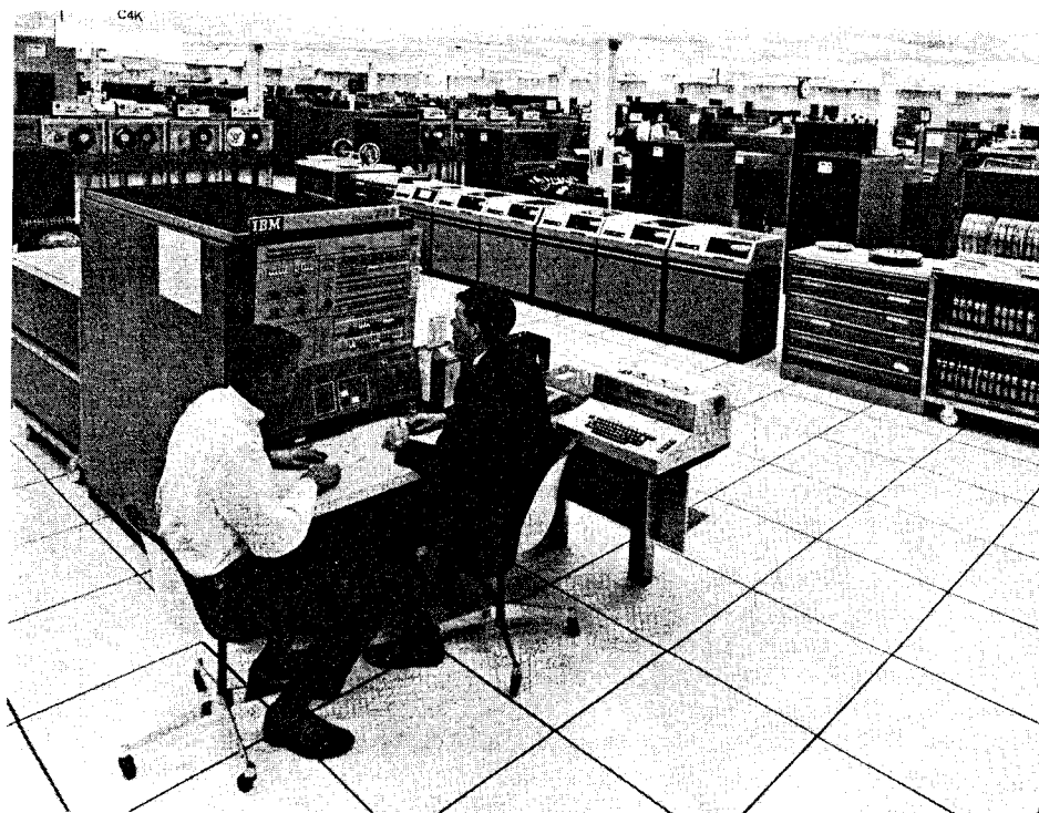
The System/360 Model 40 was introduced on April 7, 1964, and had a cycle time of 625 ns and 256 kbytes of main memory.
