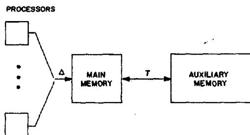
FIG. 1. Basic system hardware
