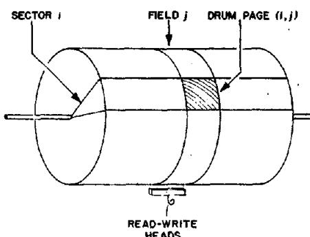
FIG. 16. Layout of paging drum
