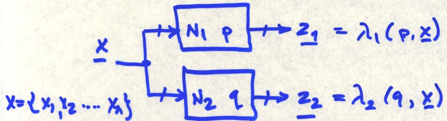
$$\underline{z}_1 = \underline{z}_2 \quad \forall \underline{x} \Rightarrow \text{then } p \equiv q$$
