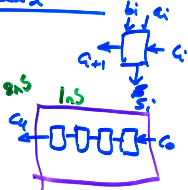
$$C_4 = \underbrace{g_3 + P_3 g_2 + P_3 P_2 g_1 + P_3 P_2 P_1 g_0}_{G} + \underbrace{P_3 P_2 P_1 P_0 \cdot C_0}_P$$
