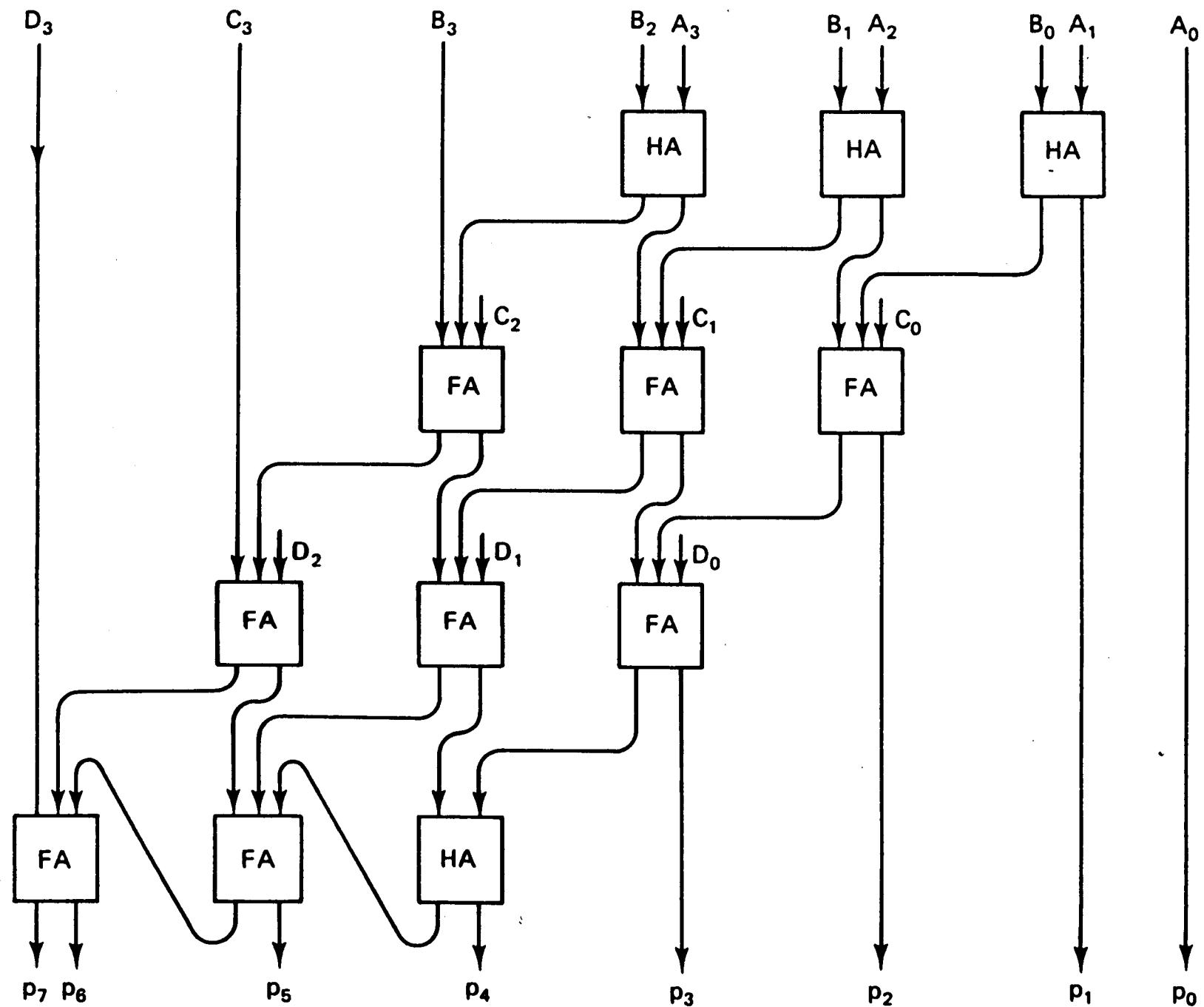
**Figure 4.4** Array of half-adders and full-adders for 4-bit  $\times$  4-bit multiplication.
